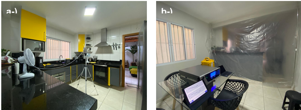
Figure 3. SP_CASA01: Example of kitchen preparation for sampling: a-) Kitchen Dimensioning and Initial Preparation; b-) Sealed or closed to begin the "Steady-State Off".
