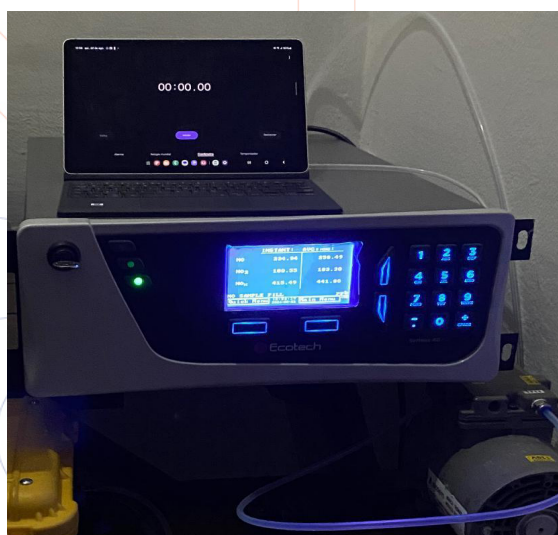
Figure 6. Analyzer Serinus 40 (Ecotech) for measurements NO, NO 2 and NO x .
